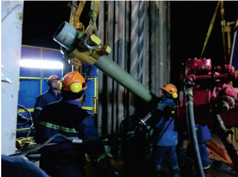
The elevator is attached to the casing.
