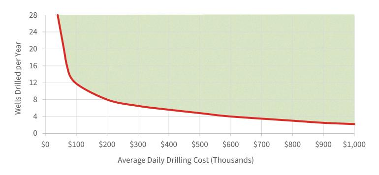
Drilling campaigns that fall above the business case frontier (illustrated by the shaded green area above the red line) are likely to see **net cost savings of over \$1,000,000** across a three year period from the use of Wired Drill Pipe.
