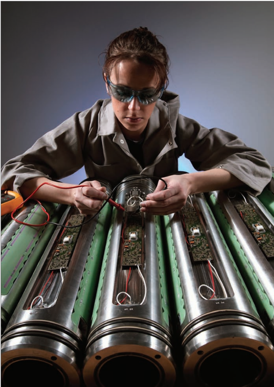
Using a downhole broadband network like The IntelliServ Network to take along-string measurements holds enormous potential, NOV IntelliServ believes. Above, electronics in the link subs get checked before being assembled into the pipe.
