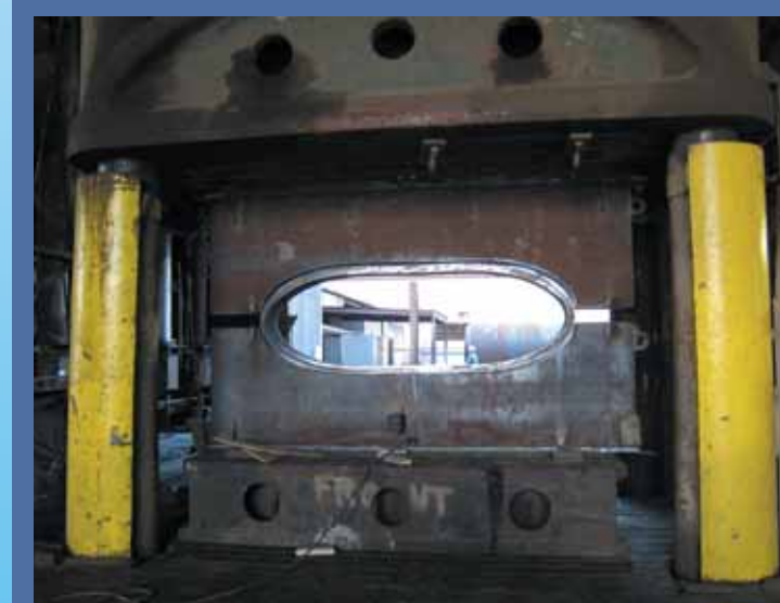
Unique to Ameron: Die Pressed Door Frames - Specialty 5,000 Ton Press
