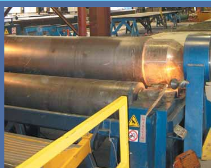
1 of 2 - New 4-roll Faccin 70 mm Bending Rolls situated for efficient material flow.
