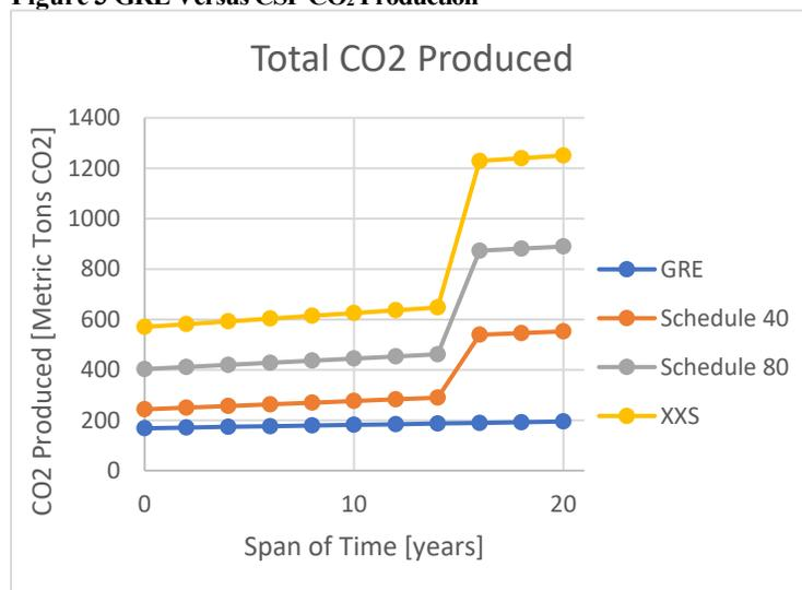
This is due to the limited life of carbon steel (e.g., in corrosive environments). Because CS pipe systems will need to be replaced at least once before the end of the field life, there are higher operating
