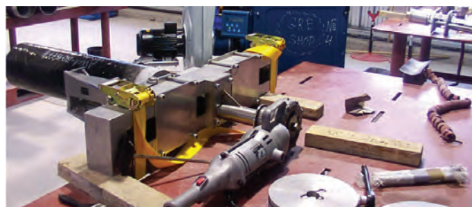
Pipe shaver to shave pipe spigot
