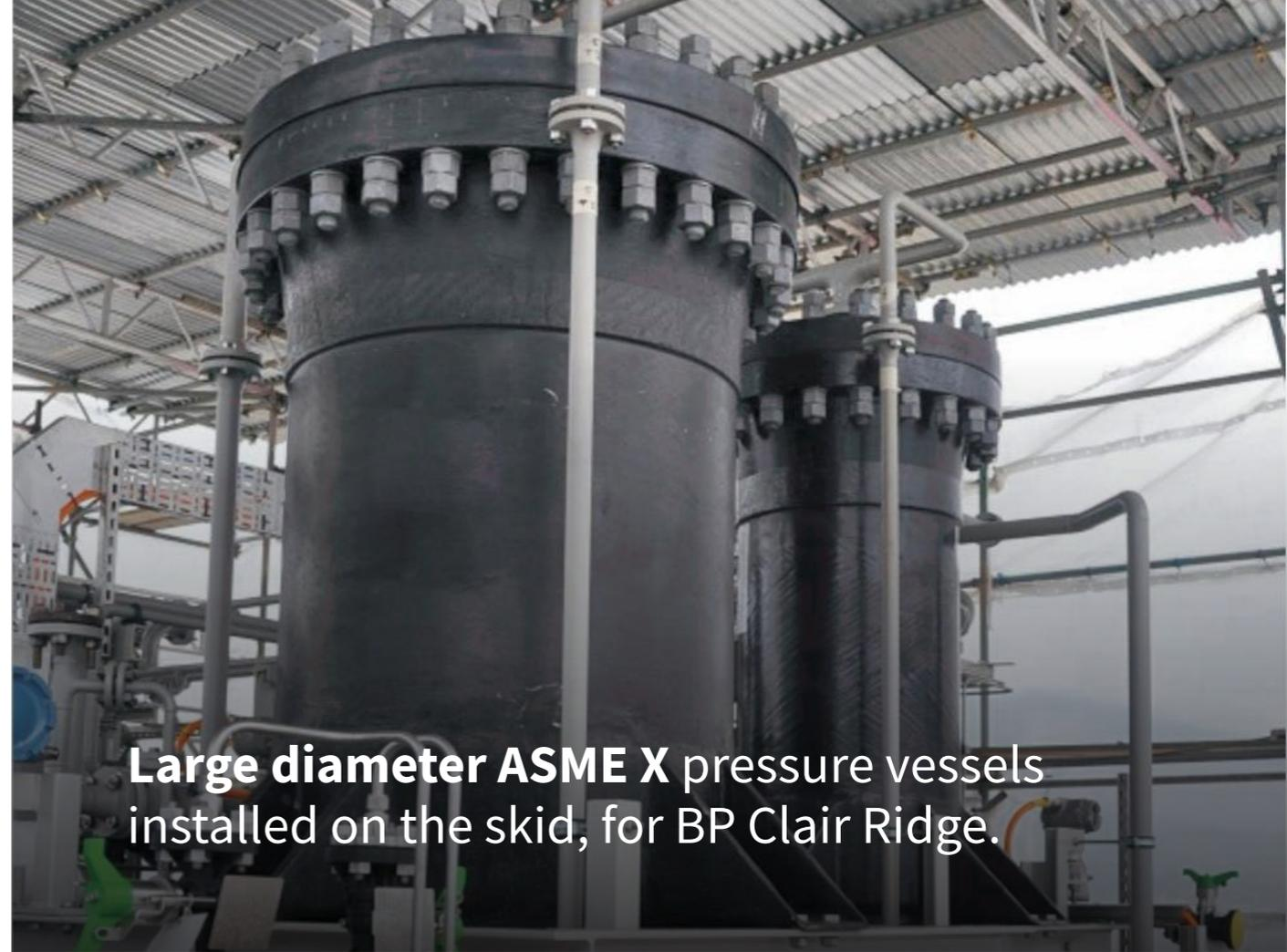
**Large diameter ASME X pressure vessels installed on the skid, for BP Clair Ridge.**
