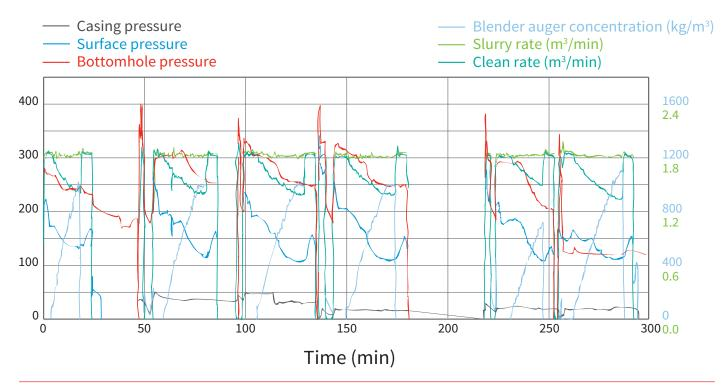
Figure 3. This graph provides a summary of multistage stimulation using the BPS and cup-to-cup tools, demonstrating the consistency and effectiveness of the system.
