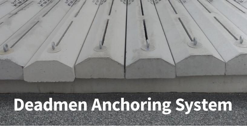
Fiber Glass Systems offers pre-fabricated deadmen anchors and turnbuckles for all Containment Solutions™ single-wall, double-wall and triple-wall underground fiberglass storage tanks. Deadmen anchors provide a means to prevent installed tanks from floating out of the ground when the tank installation is subject to ground water. Deadmen anchors are just as effective at preventing tank flotation but cost less than a concrete pad under the tank.
