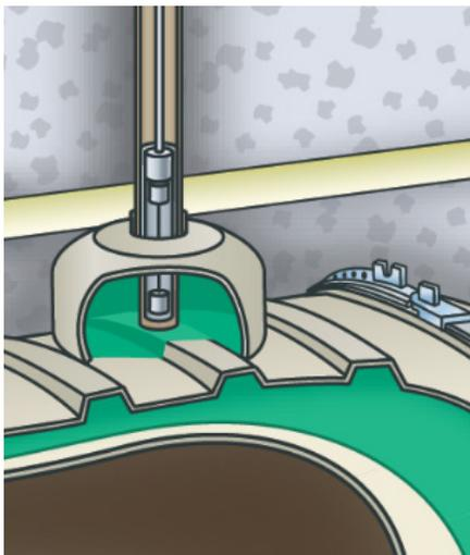
Hydrostatically Monitored Double-Wall Fiberglass Tank Sump
