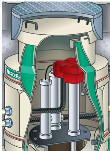
Hydrostatically Monitored Double-Wall Fiberglass Tank
