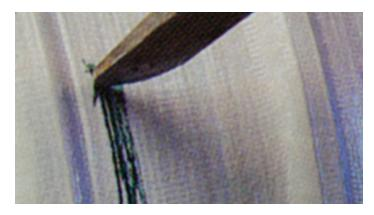
Transport or handling damage is instantly identifiable by a contrasting colored brine solution, an exclusive feature of a Containment Solutions™ hydrostatically monitored double -wall tank.
