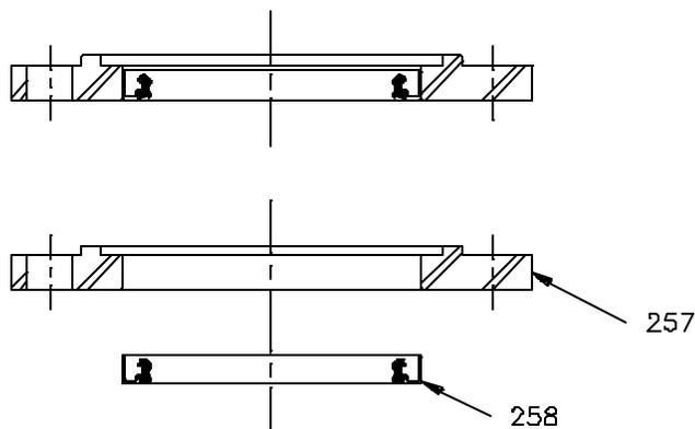
Figure 4: Lower Bearing Cap Assembly [256]
