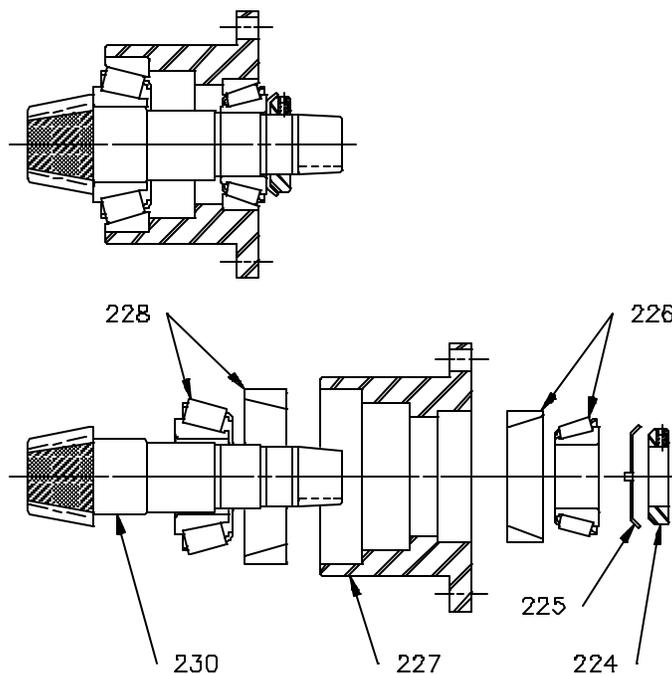
Figure 13: Spiral Bevel Pinion Cartridge Assembly [223]
