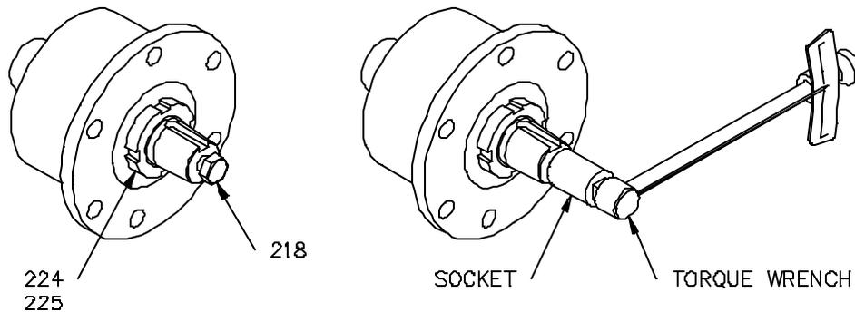
*Figure 14: Torque Reading*
