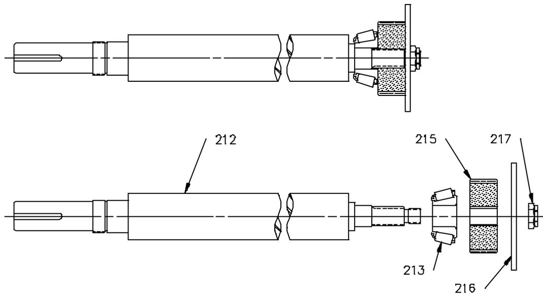
Figure 9: Input Shaft Assembly [211]
