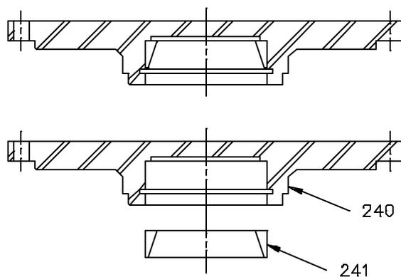
Figure 10: Upper Bearing Cap Assembly [239]
