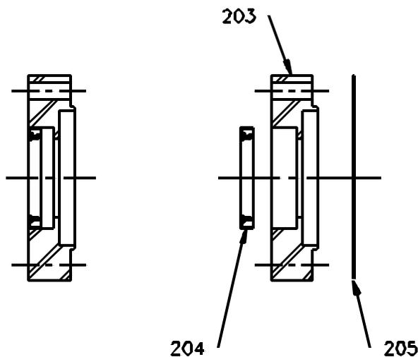
Figure 8: Input Shaft Bearing Cap Assembly [201]
