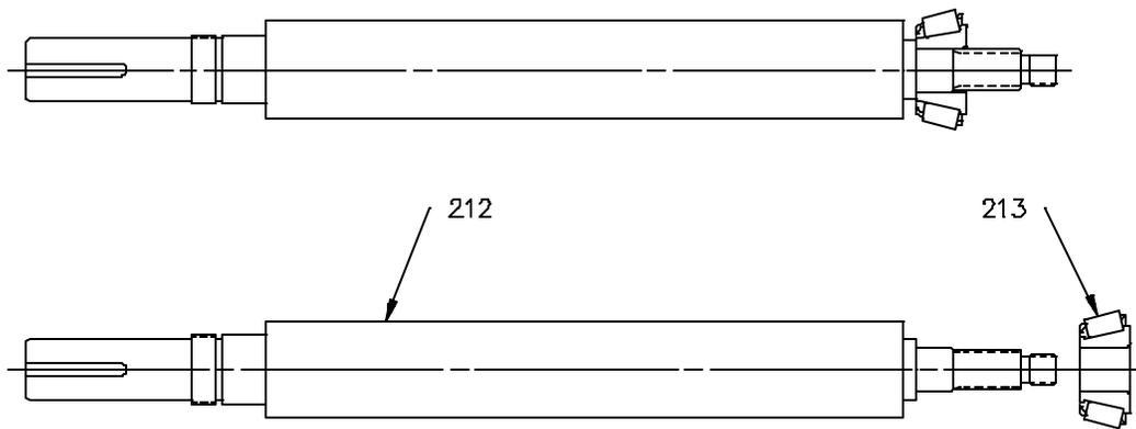
Figure 5: Input Shaft Assembly [211]
