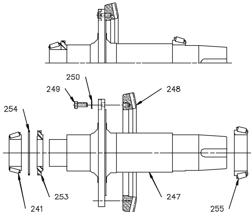
Figure 12: Output Shaft Assembly [246]
