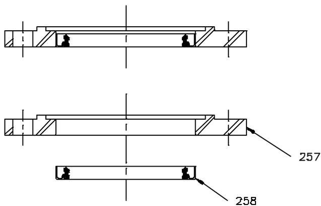
Figure 11: Lower Bearing Cap Assembly [256]
