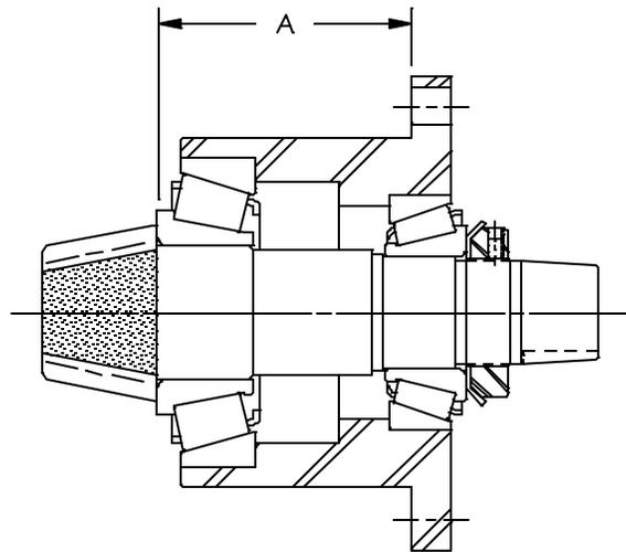
Figure 15: Cartridge Measurement
