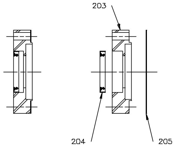
Figure 6: Input Shaft Bearing Cap Assembly [201]
