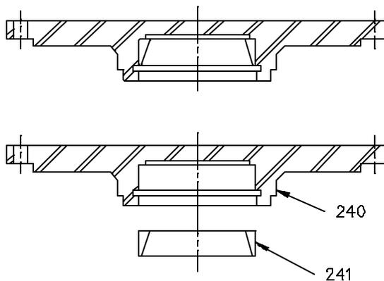
Figure 3: Upper Bearing Cap Assembly [239]
