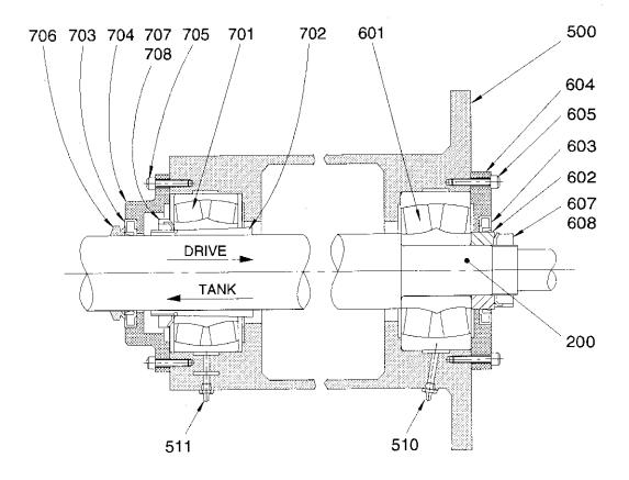
Figure 32: MD Agitator Assembly - Type 4
