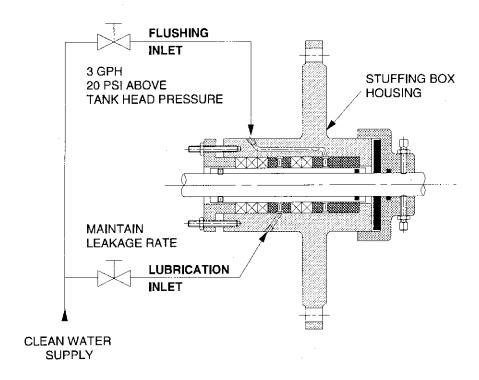
Figure 20: Type DL Stuffing Box Lubrication
