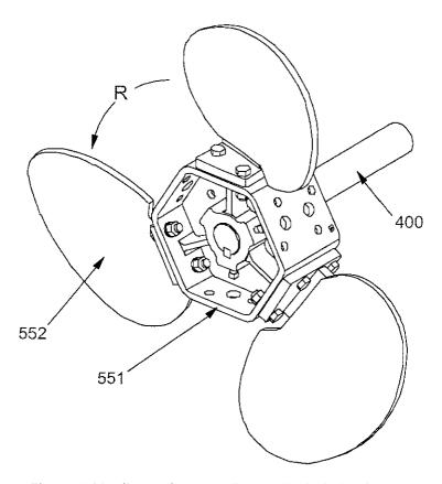
Figure 1 Maxfio Mark II Impeller (Bolted Blade Shown)
