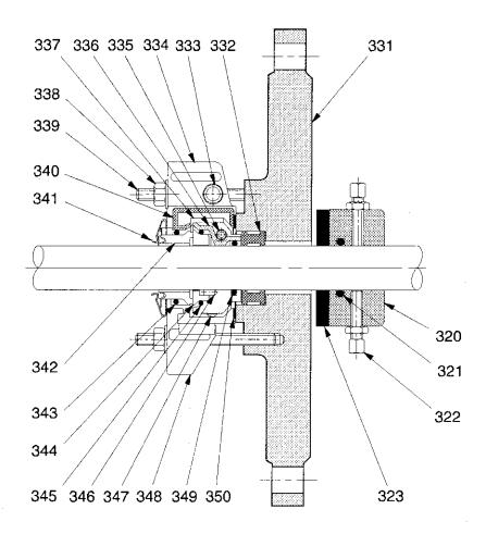
Figure 26: Type OM Split Mechanical Seal
