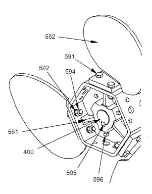
Figure 2 Maxflo Mark II with Bolted Blades 25" Through 87" Diameter
