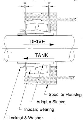
Figure 33: Inboard Bearing Position
