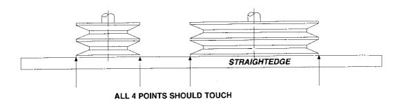
Figure 17: Sheave Alignment
