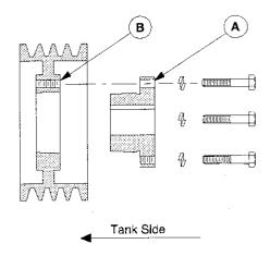
Figure 16: "Flange-Out" Mounting
