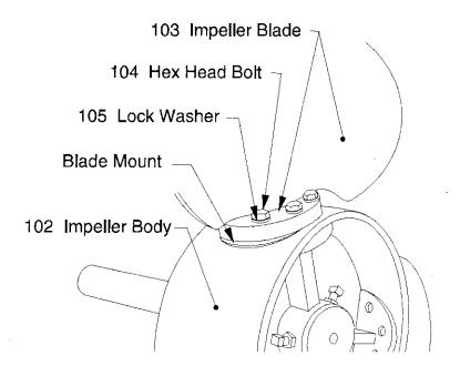
Figure 10: Removable Blades - Maxflo Mark II Impeller
