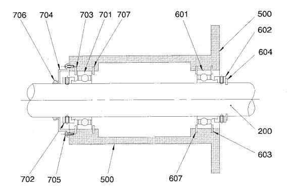
Figure 29: MD Agitator Assembly - Type 2
