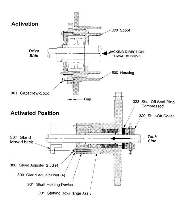
Figure 23: Tank Shut-Off Activation Feature
