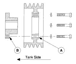
Figure 15: "Flange-In" Mounting
