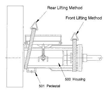
Figure 2: Lifting Lug Location
