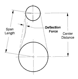
Figure 18: Belt Tensioning
