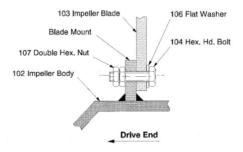
Figure 14: Removable Blades Maxflo Mark III Impeller
