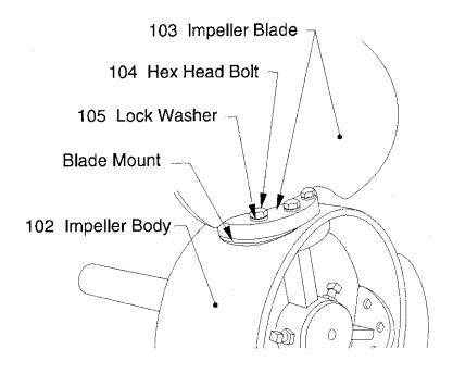
Figure 8: Maxflo Mark II Impeller
