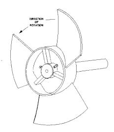
Figure 11: Maxflo Mark III Impeller
