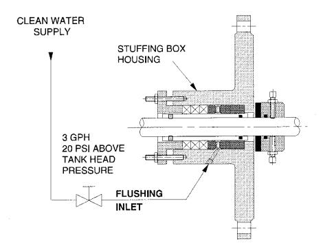
Figure 19: Type L Stuffing Box Lubrication
