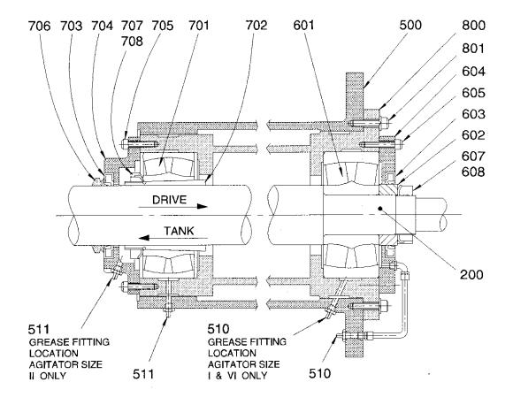
Figure 31: MD Agitator Assembly - Type 3
