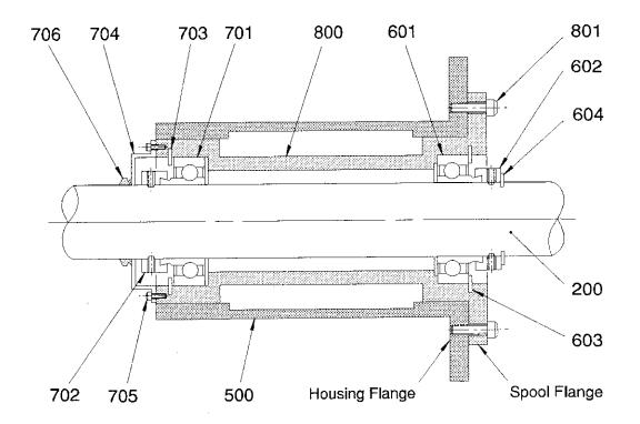
Figure 28: MD Agitator Assembly - Type 1
