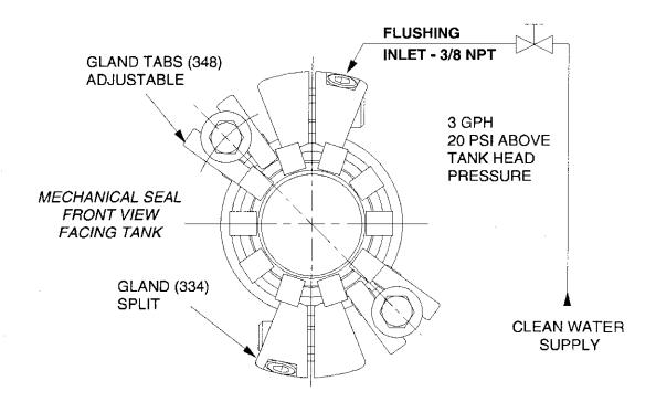
Figure 21: Type OM Mechanical Seal Lubrication
