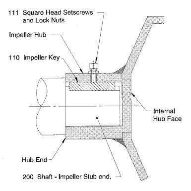
Figure 13: Impeller Hub Attachment - Closed-Body Design
