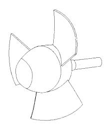
Figure 12: Maxflo Mark III Impeller with Optional Nose Cone
