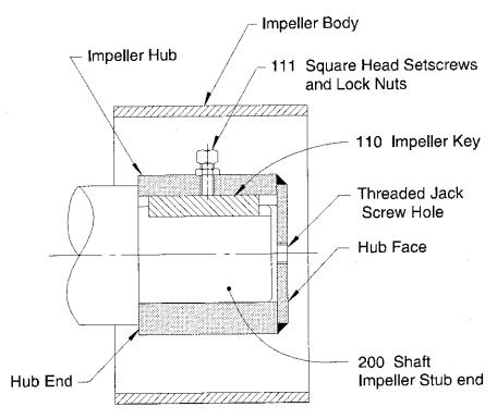
Figure 9: Impeller Hub Attachment - Open Body Design
