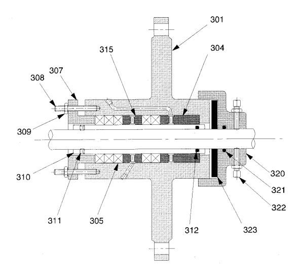
Figure 25: Type DL Stuffing Box
