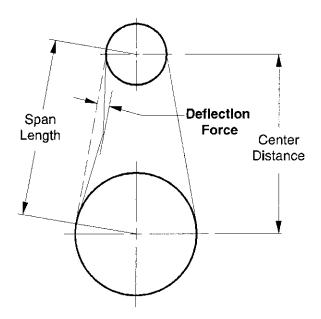
Figure 34: Belt Tensioning
