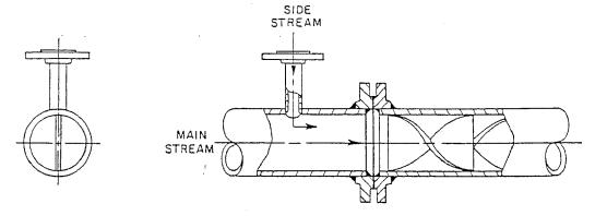
The sidestream introduction point should be as close as possible to the first element, usually no more than 1-2 pipe diameters upstream. Introduction should be in the center of the pipe and parallel to the leading edge of the first element as shown above. The sidestream velocity should be equal to approximately twice the mainstream velocity. Where the above component ratios are exceeded, for either blending or dispersion, Method 2 injection is preferred.
