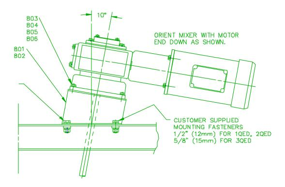
Figure 1.1: Angle Riser Mounting
