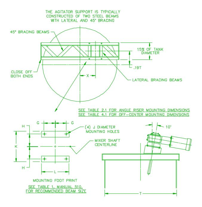
Figure 1.2: Angle Riser Mounting
