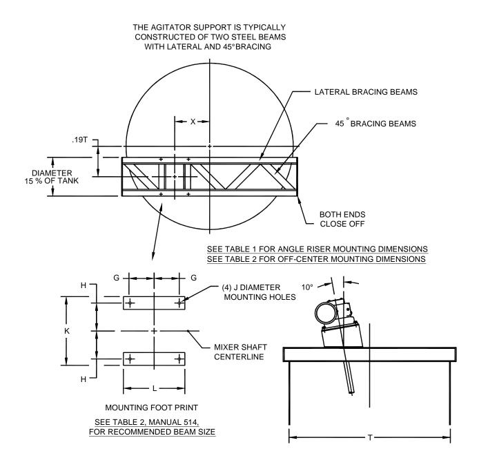
Figure 2: Angle Riser Mounting – Orientation
