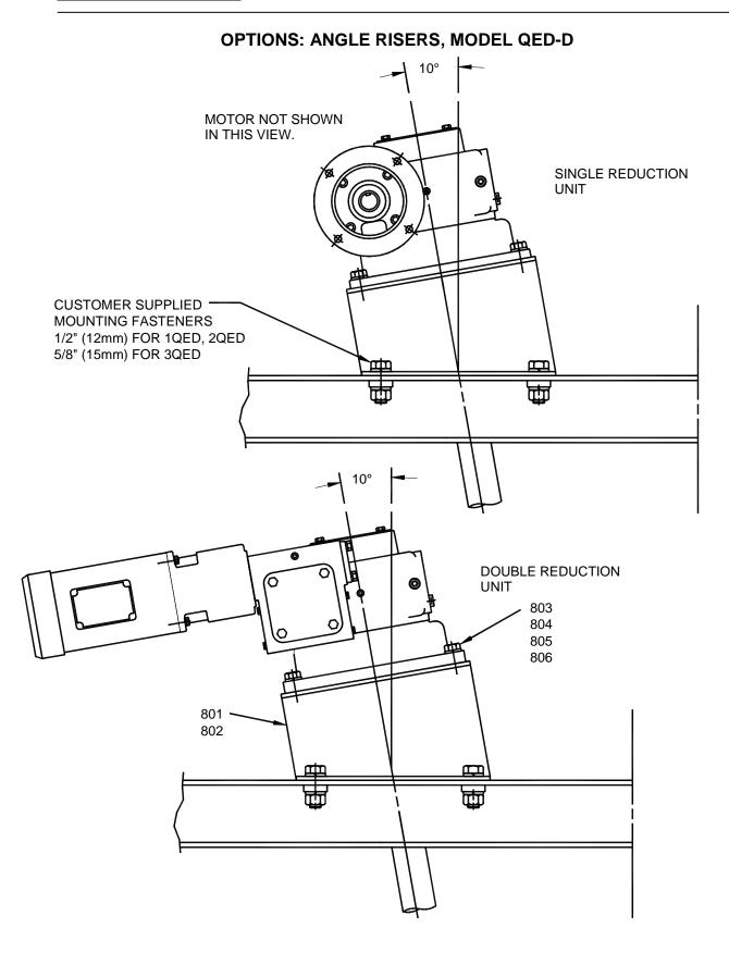
Figure 1: Angle Riser Mounting
