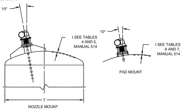
Figure 4: Closed Tank Angle Mounting - Orientation
