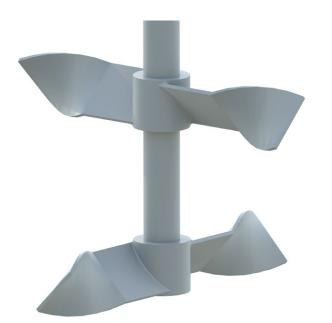
The JT-2 impeller is used for superior blending in transitional flow. High viscosity and non-Newtonian fluids make blending much more challenging. This impeller is used after conventional turbines have lost efficiency due to viscous effects and before the need for close clearance impellers.
