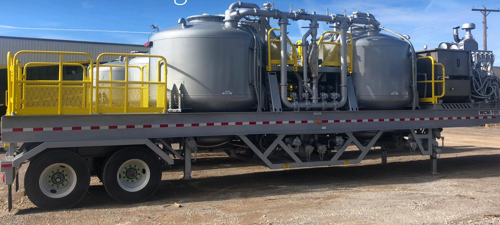
Our mixing-displacement manifolds have a 100-bbl capacity and are offered in three different centrifugal pump configurations.
