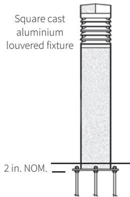
(4) 1/2 in. X 12 in. Galv. Steel Anchor Bolts W/ Washers Astm F1554 Grade 36
