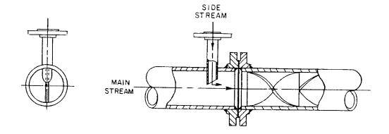
The smaller stream should be injected into the main flow. The injector tip of the minor component should be in the center of the pipe and as close to the leading edge of the first element as possible, ideally less than one pipe diameter. Injection should be parallel to the leading edge of the first element as shown above. The sidestream velocity should be approximately two times the mainstream velocity, regardless of component viscosities.
