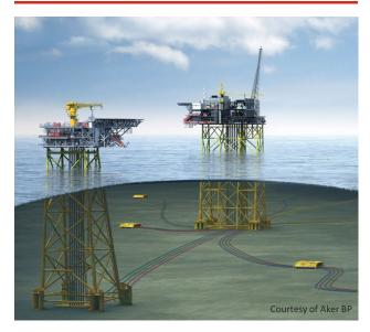
Customer/End User: Aker Solutions/Aker BP Solution: Selected for FEED with a concept for a 138,500 BPD HVAC enclosed single-lift module consisting of UF, SRU feed pumps, SRU, Membrane Deaeration with PSA nitrogen/vacuum systems, CIP, and chemical dosing skid.
