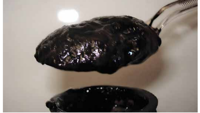
Figure: Oily sludge removed from heater-treaters.
