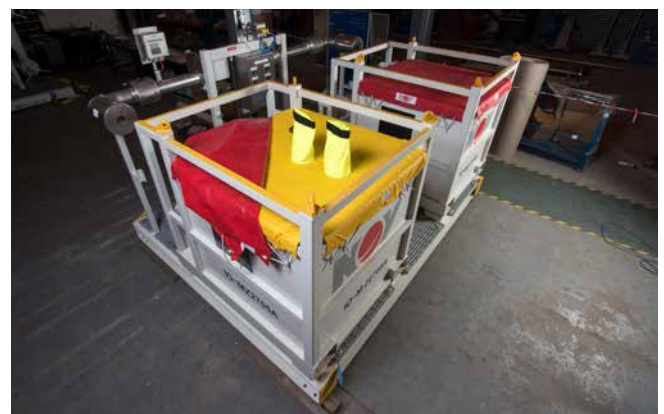
Figure: Sand bagging station and transportable containers
