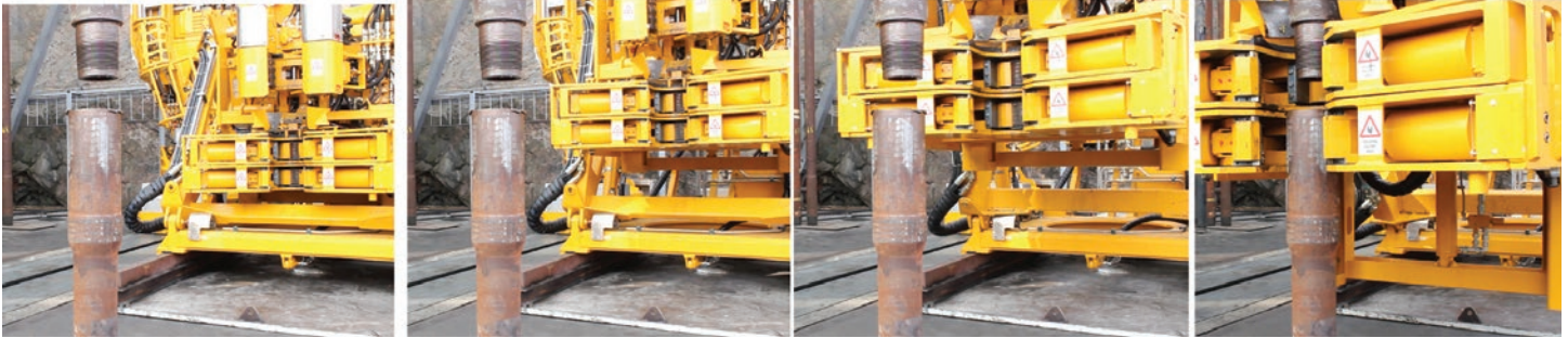
Figure 2. ARN-200 iron roughneck trajectory optimization during testing and calibration
