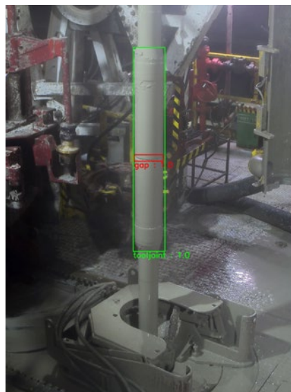
Fig 1. Camera technology analyzing tool joint and stickup height
