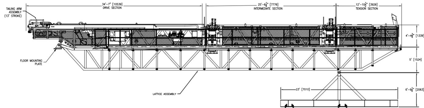
The Pipe Transfer Conveyor (PTC-LD) is a light duty conveyor with an attached Tailing Arm Assembly. The PTC transports drilling tubulars between their storage location on the main pipe deck and well-center without manual intervention from the rig crew. It can be remotely operated from the rigs main control cabin through integrated controls or operated locally from a local control station. The PTC has two main sections: Conveyor & Tailing Arm Assembly.
