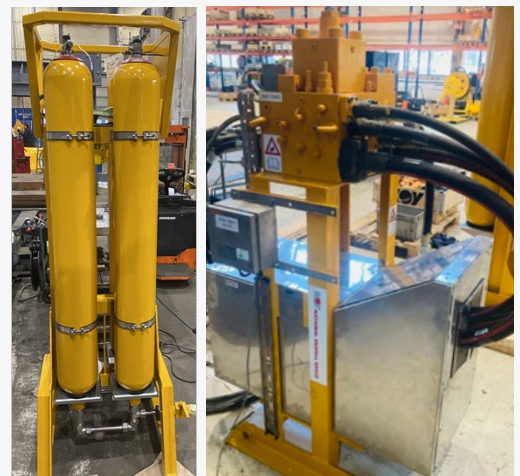
Accumulator skid and booster skid components of the EcoBooster.
