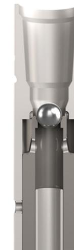
With pumps off, the tool returns to reset position. Even with the ball on seat, the MOCS G2 is designed to allow the drill stem to drain while tripping pipe.
