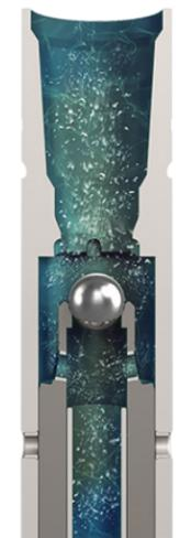
Once in non-bypass mode with the ball on the seat, the tool routes flow back to the bit to continue circulation through the entire BHA.
