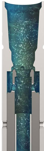
Run in hole position with open through bore.
