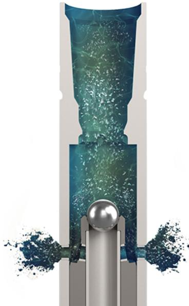
Pump pressure forces the piston valve down, opening the ports to the annulus and closing off flow through sensitive BHA components.
