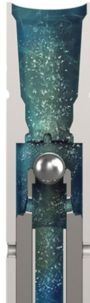
Once in non-bypass mode with the ball on the seat, the tool routes flow back to the bit to continue circulation through the entire BHA.
