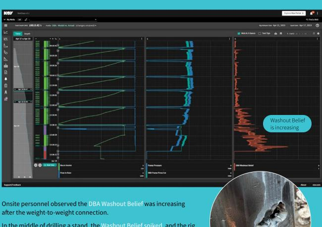
In the middle of drilling a stand, the Washout Belief spiked, and the rig team decided to trip out of the hole to assess the potential issue.
