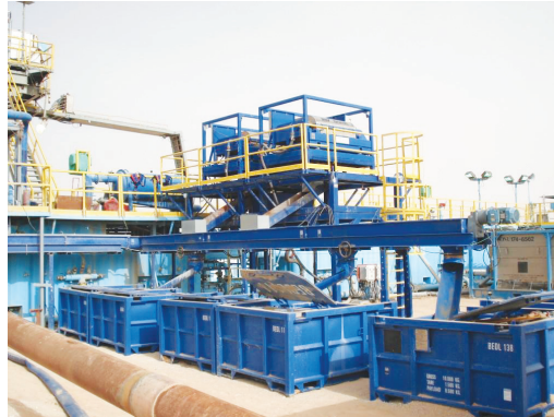
The FluidControl closed loop solids control and high thermal desorption system on location in North Africa.
