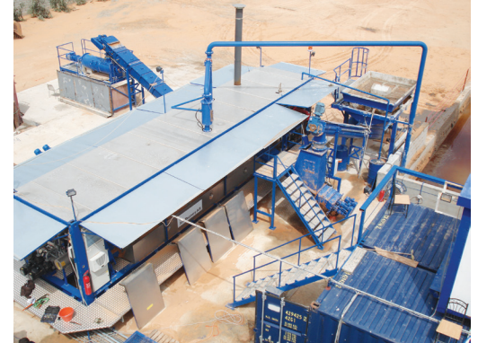
The FluidControl closed loop solids control and high thermal desorption system on location in North Africa.
