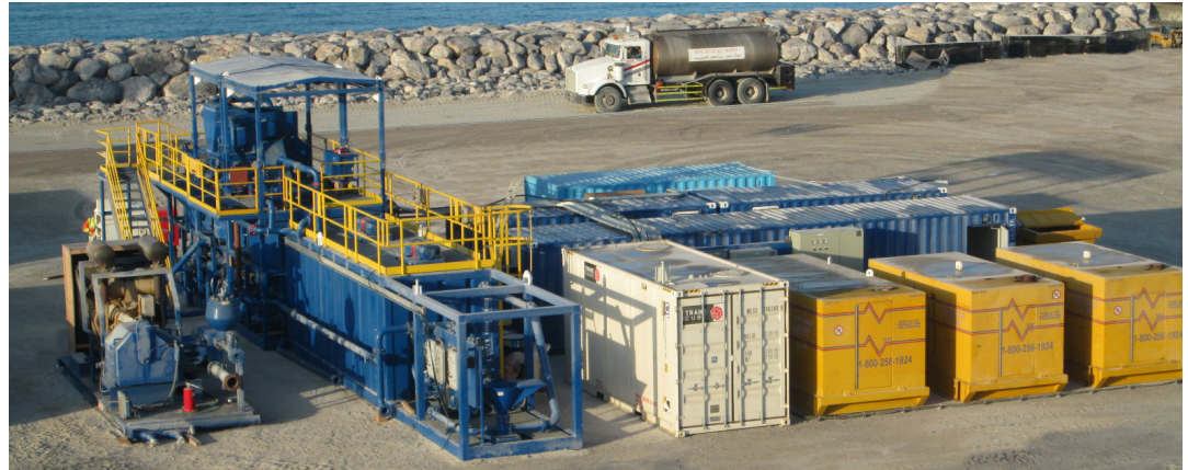
Based on an artificial island in the Arabian Sea, the FluidControl CRI configuration is unique in that all components, including injection and grinding pumps, high-pressure piping, the slurrification unit and classifying shakers were custom-designed and manufactured by multiple NOV divisions. Installation of a similar CRI setup is underway on the second island awarded in the initial contract.
