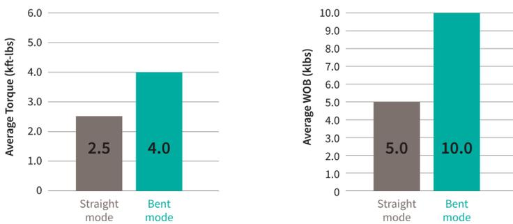
Figure 1. SelectShift rotary drilling comparison (ROP fixed).
