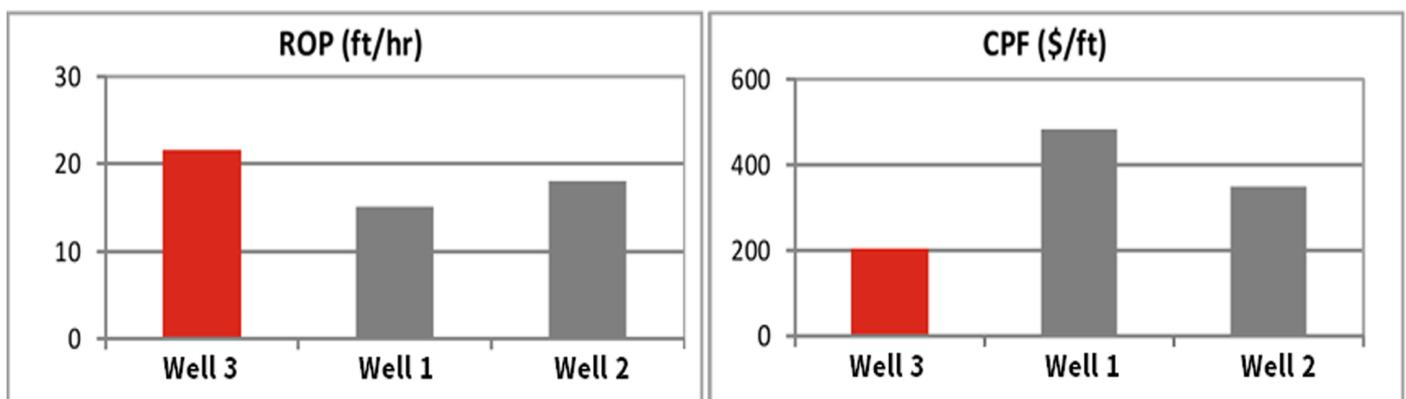
**Figure 3.** On the first offset well, ROP was 15.1 ft/hr, and on the second, it was 18 ft/hr. Based on the number of bits used and time downhole, the CPF for the first well was 483.3/ft, and it was 349.3/ft for the second. With the addition of the Agitator system and MOCS, ROP increased to 21.5 ft/hr, and CPF decreased significantly to 204 ft/hr.
