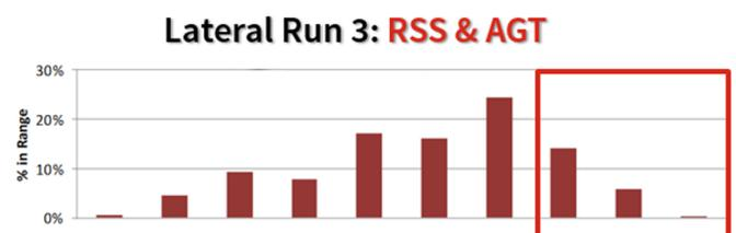
**Figure 2.** The run with the RSS spent 50% of the time within the weight range of 23 - 28 000+ lb compared to 20% of the time spent in the same range by the Agitator and RSS combination in the deeper and longer interval, clearly showing that the system improved torque and drag response.
