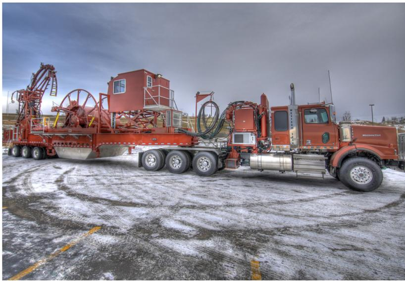
**Figure 2.** The new coiled tubing unit, designed to allow rapid change-out of suspension/axle groups to enable movement between countries.
