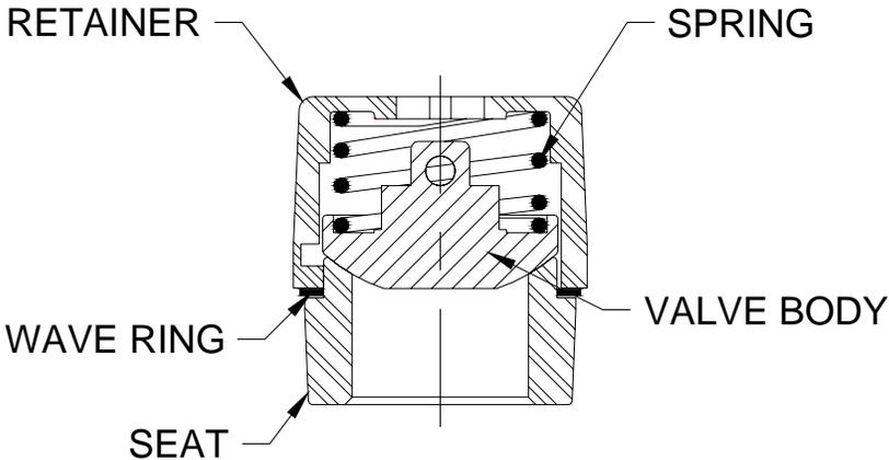
**SPHERICAL VALVE ASSEMBLY**
