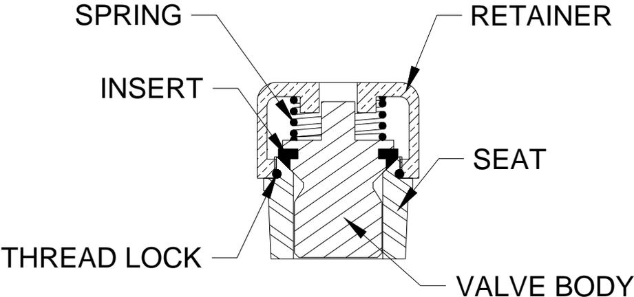
**SEVERE DUTY VALVE ASSEMBLY**
