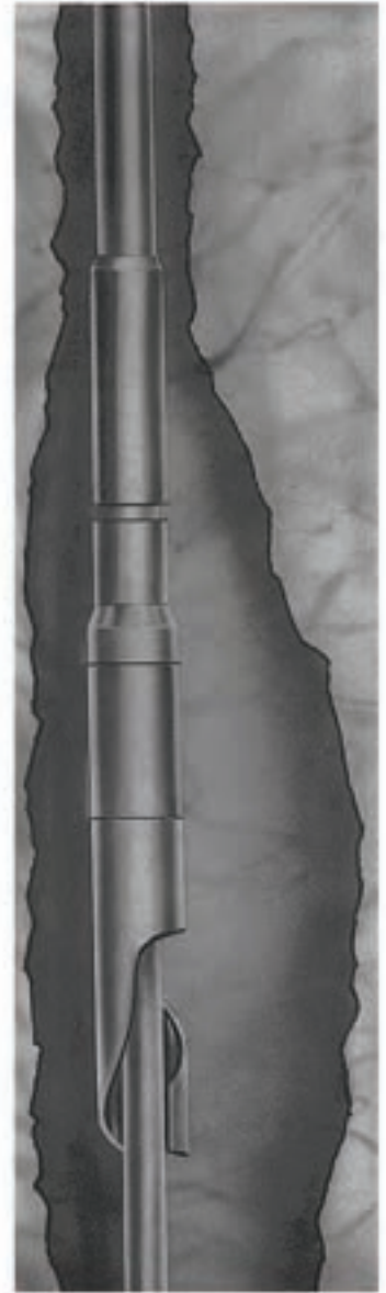
After Contacting the Fish, Ready for Retrieval
