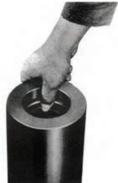
Figure 7 Insert one edge in groove. Then insert the opposite edge and press down until entire ring is in place.
