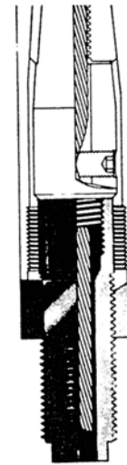
Extractor Tool Shown in Position
