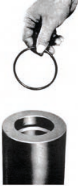
Figure 10 j. Figure 10 shows o-ring packing before installation.
