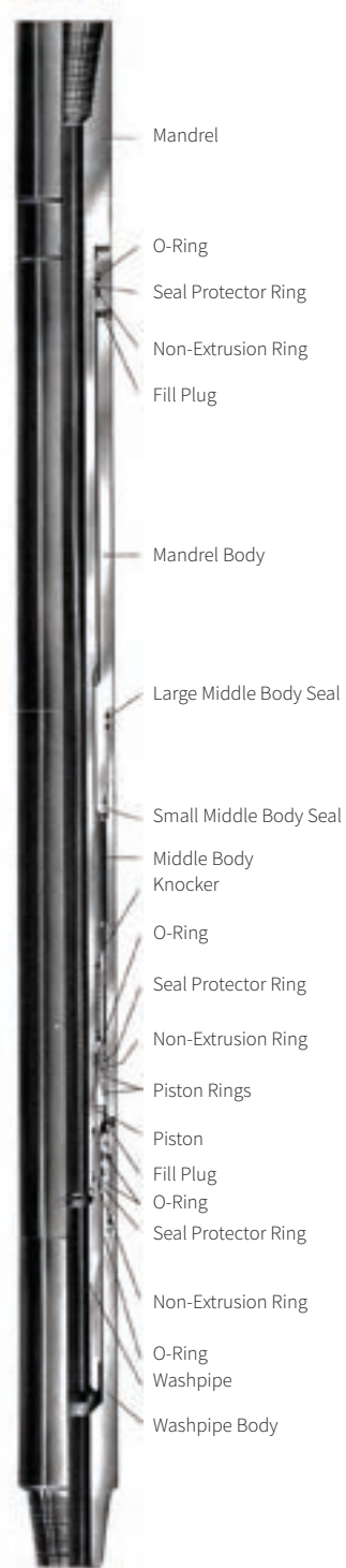
Figure 5 Integral Mandrel Jar
