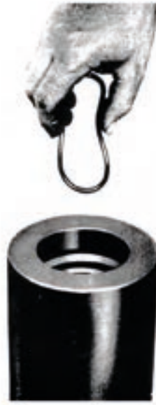
Figure 11 k. Bend o-ring as shown to insert in groove.
