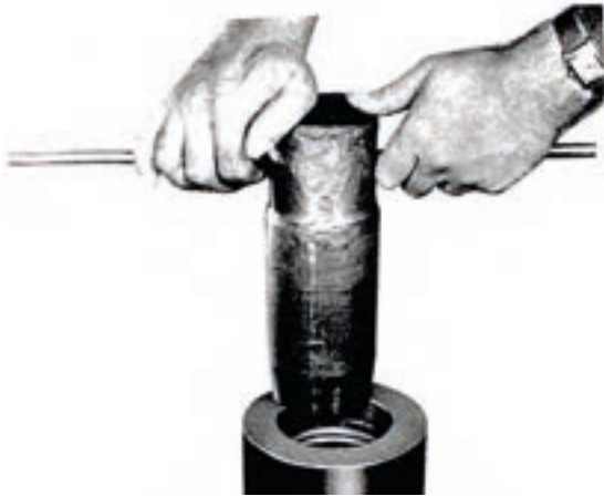
Figure 15 b. Insert the setting tool as shown, using any convenient rod or bar to hold tool.
