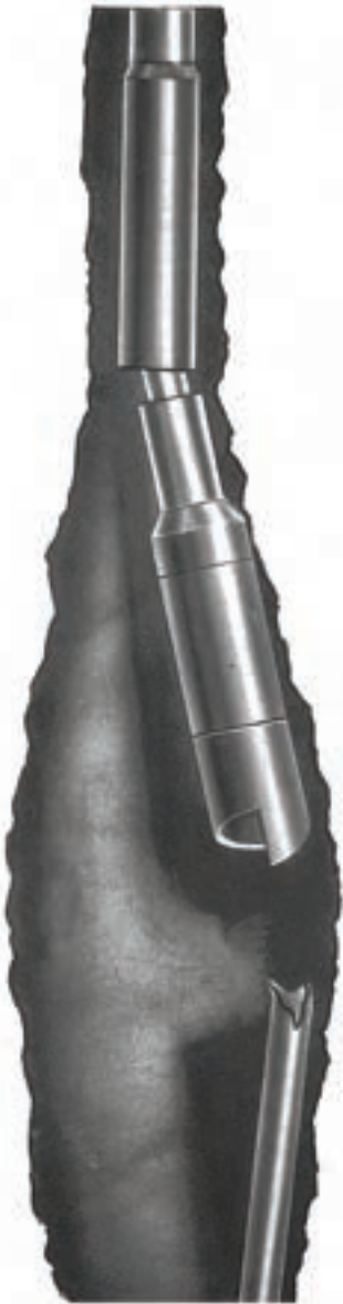
Knuckle Joint Positioning Overshot Being Lowered to Engage Fish
