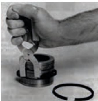
Figure 7 Piston ring removal
