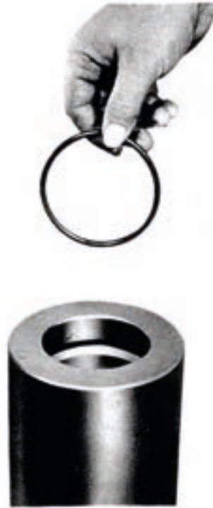
Figure 18 O-ring packing before installation.
