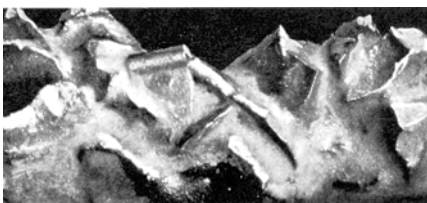
A macro-photograph of a portion of an Itcoloy Rod showing the concentration of tungsten carbide particles imbedded in the nickel-silver alloy matrix.
