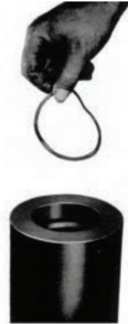
Figure 6 Bend the ring until it is small enough to allow entry into bore.
