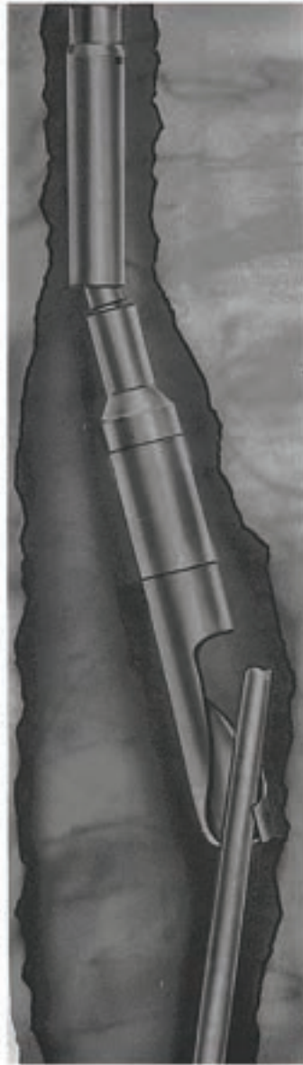
Bowen Lebus Knuckle Joint with Overshot and Wallhook Guide Contacting Fish in a Cavity
