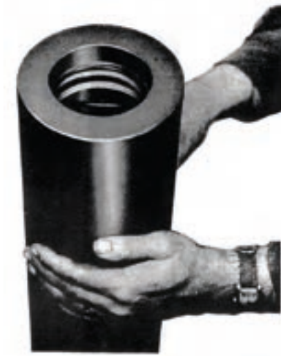
Figure 12 l. Insert o-ring between seal protection rings in each groove.
