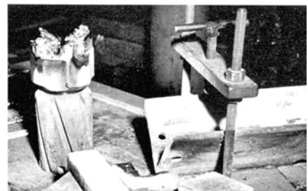
The Junk Mill has been removed from the fixture and is positioned for finishing the bottom face of the mill with Itcoloy. Note that all of the cutting faces conform to the shape of the carbon block mold.
