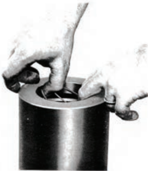
Figure 3 Place edge of ring opposite the split into the lower groove and spread from center toward ends. Be sure beveled side of ring matches beveled groove side.
