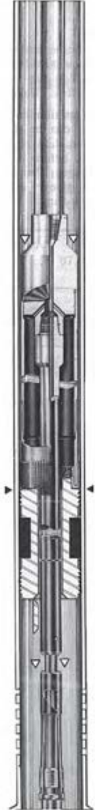
Mill Away Slips and Sealing Element
