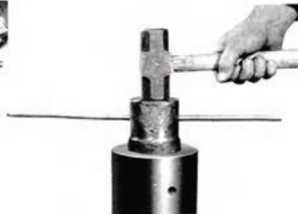
Figure 24 Drive in as shown and tap several times around the periphery of the tool to set the rings. Continue until both ring assemblies are seated. Then remove the tool and continue assembly of the sub.
