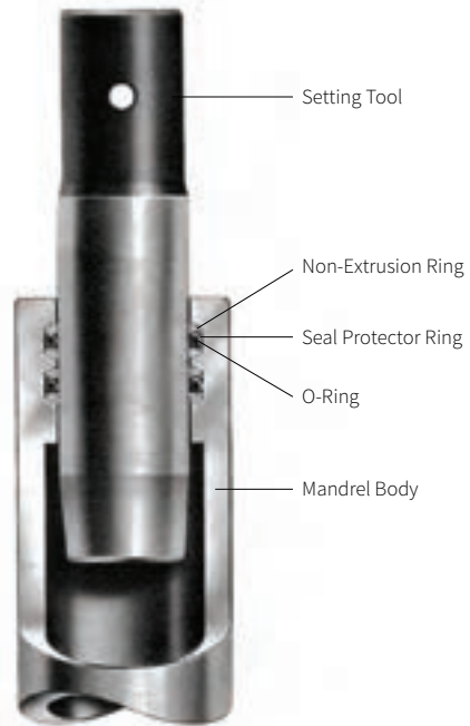
Figure 12 This illustration shows the O-ring seal assemblies in place inside the mandrel body. The setting tool is shown in position as it is being driven into the bore to conform the copper rings to the proper size. If plastic seals are used, a setting tool is not required.
