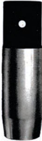
Figure 13 Use this setting tool from the service accessory kit (See page 14) to seat the ring seal assemblies after installation.
