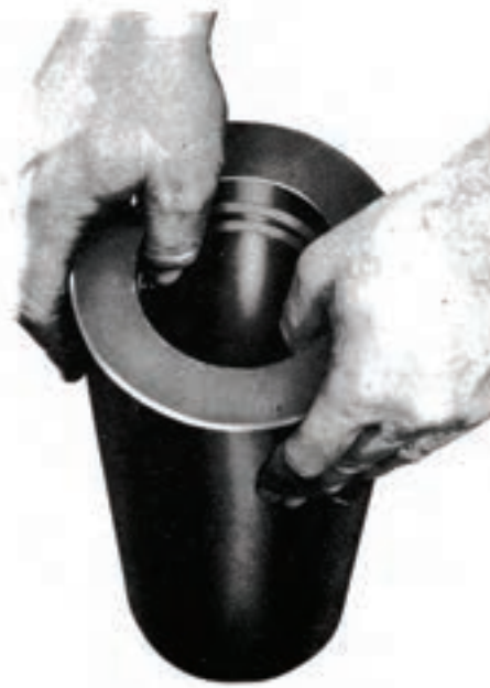
Figure 4 Using thumbs, press ring into groove until ends match up and ring is firmly seated in groove.
