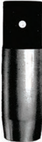
Figure 13 Use this setting tool from the accessory kit to seat the ring seal assemblies after installation. (Not required with black nylon rings.)
