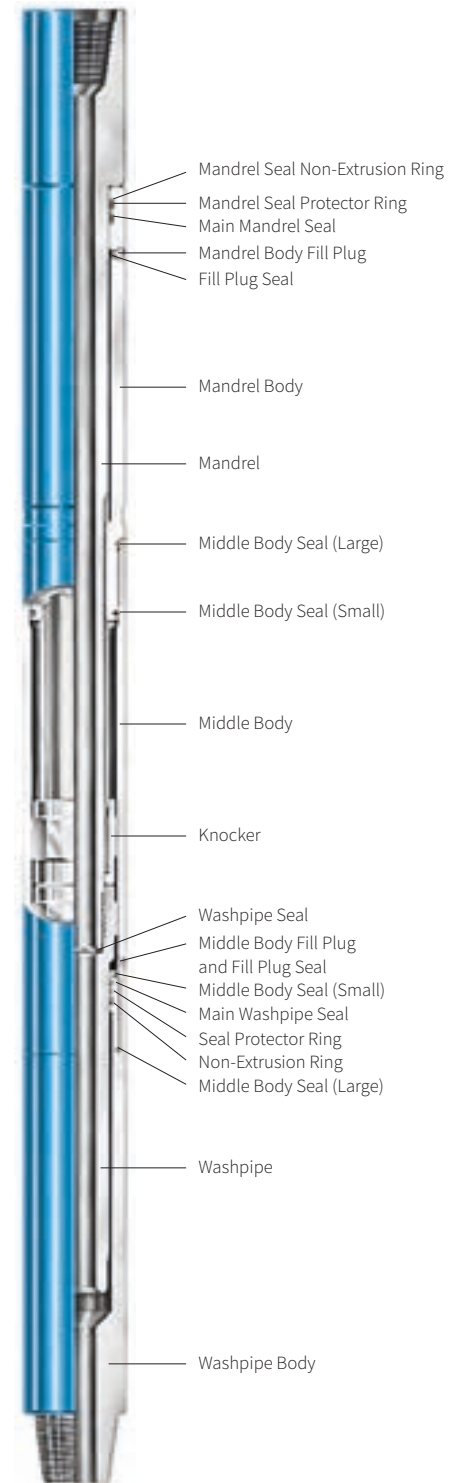
Bowen Lubricated Fishing Bumper Sub
