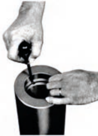
Figure 1 O-Ring Removal with Tool No.625
