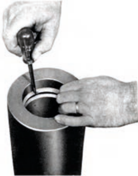
Figure 17 Use a seal protector ring Installation Tool to straighten and flatten the ring by pressing against the ring as shown.
