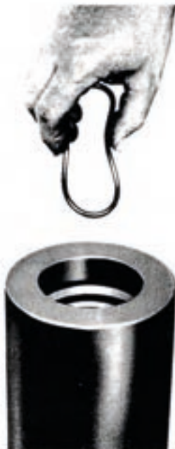
Figure 19 Bend the o-ring as shown to insert into the groove.
