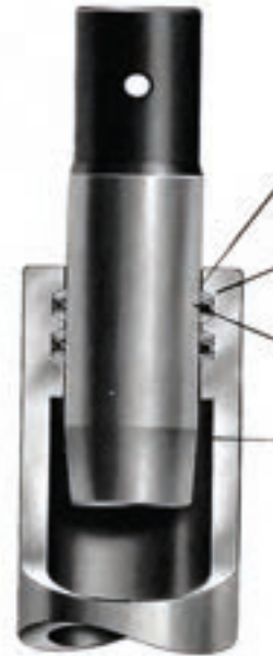
Figure 22 The above illustration shows the o-ring seal assemblies in place in the mandrel body. The setting tool is shown in position as it is being driven into the bore to conform the copper rings to proper bore size.
