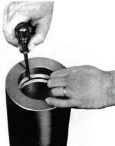
Figure 8 Use seal protector ring installation tool to straighten and flatten ring by pressing against ring as shown.
