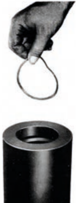
Figure 15 Bend the ring until it is small enough to allow entry into bore.
