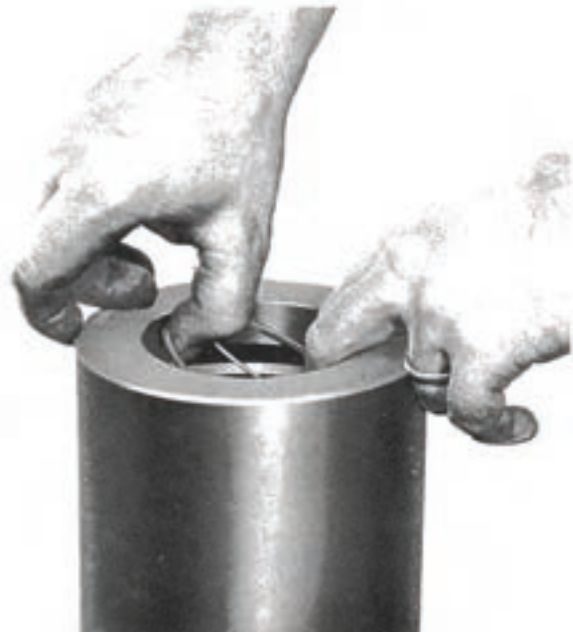
Figure 12 Place edge of ring opposite the split into the lower groove and spread from center towards ends. Be sure the beveled side of the ring matches the beveled groove side.
