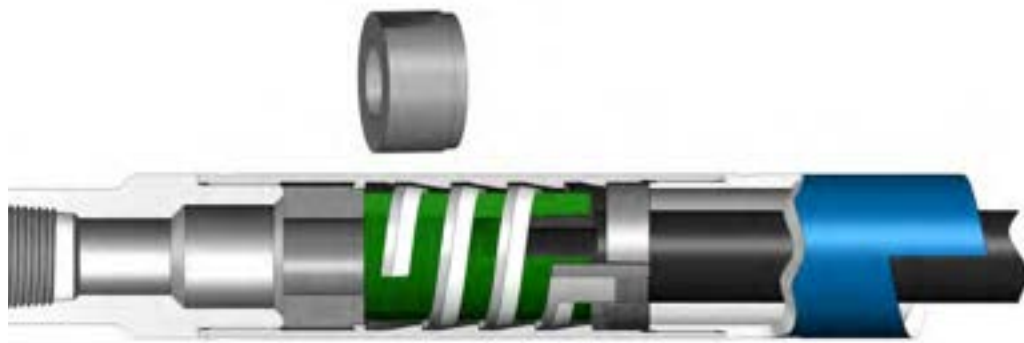
Stop Ring with Overshot and Coupling
