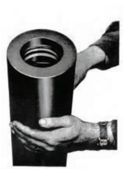
Figure 11 Insert O-rings between seal protection rings in each groove.
