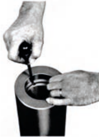
Figure 8 Seal assembly removal
