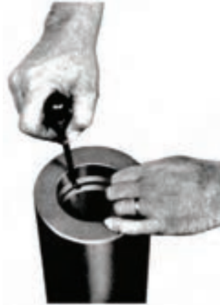
Seal Assembly Removal
