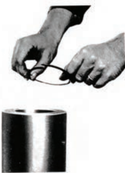
Figure 1 Hold non-extrusion ring between thumbs and forefingers as shown.
