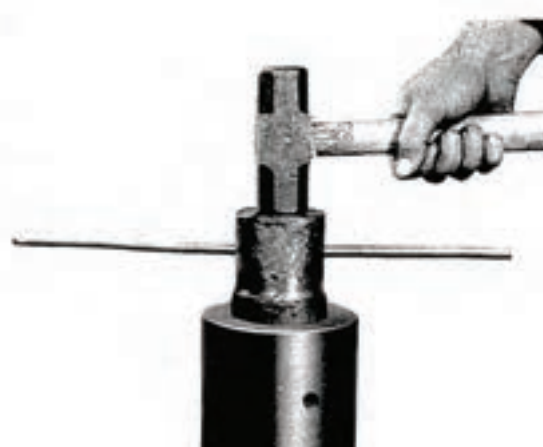
Figure 16 Drive in as shown and tap several times around the periphery of the tool to set the rings. Continue until both ring assemblies are seated. Then remove the tool and continue assembly of the sub.
