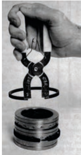
Figure 25 Piston ring installation
