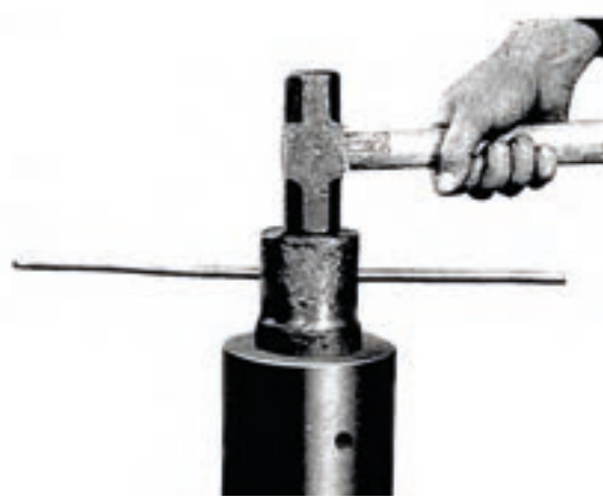
Figure 16 c. Tap several times around periphery of tool as shown to set rings. Continue until both ring assemblies are seated. Then remove tool and continue assembly.
