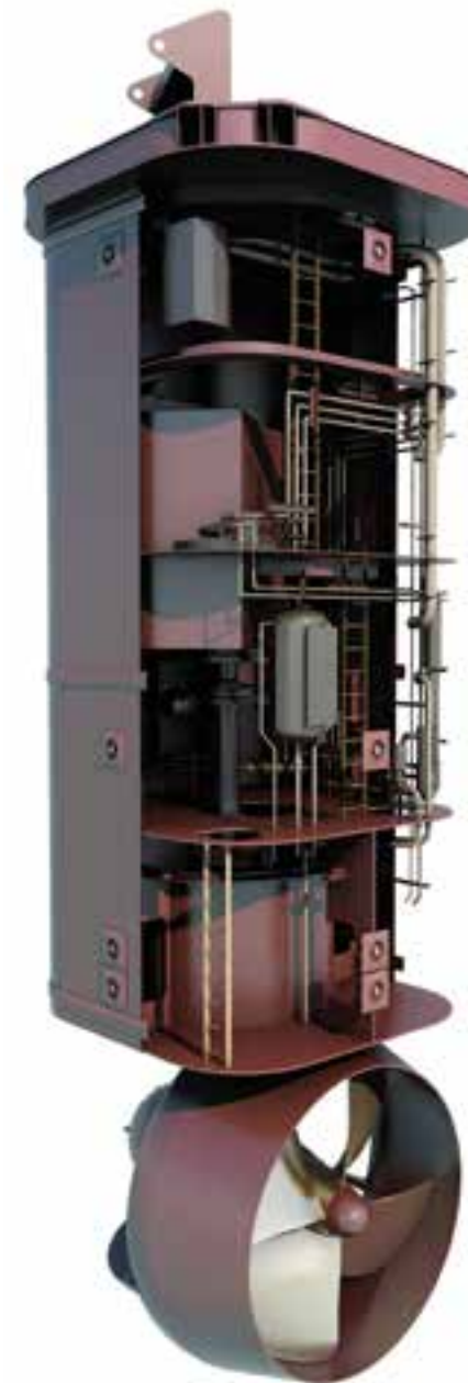
The TRS canister with the azimuth thruster machinery
