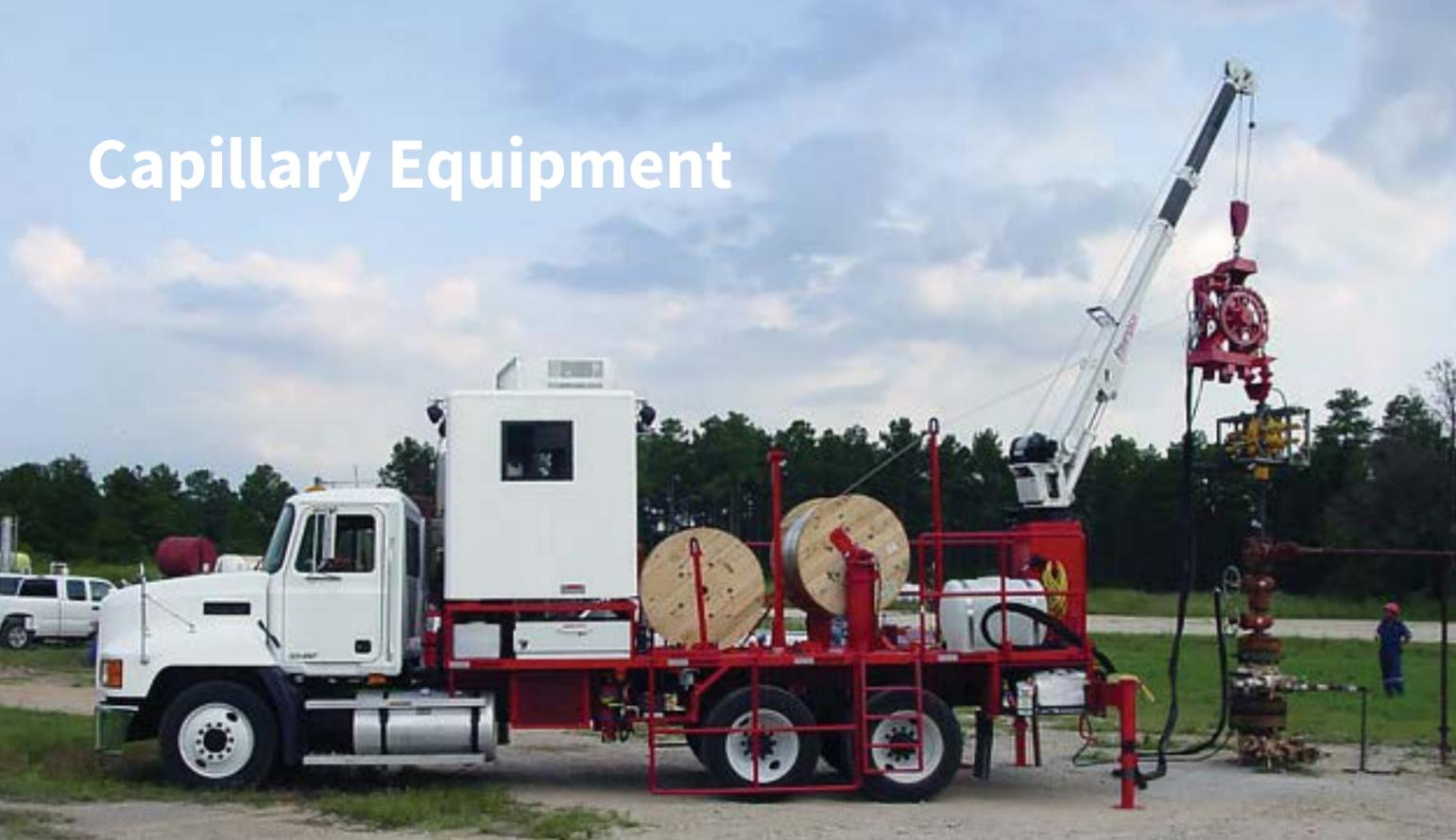
Maximize well production with our capillary tubing units. Units are engineered for precise placement of capillary string to reliably increase well productivity by treating paraffin, corrosion, scale build-up and produced water via foam-lift.
