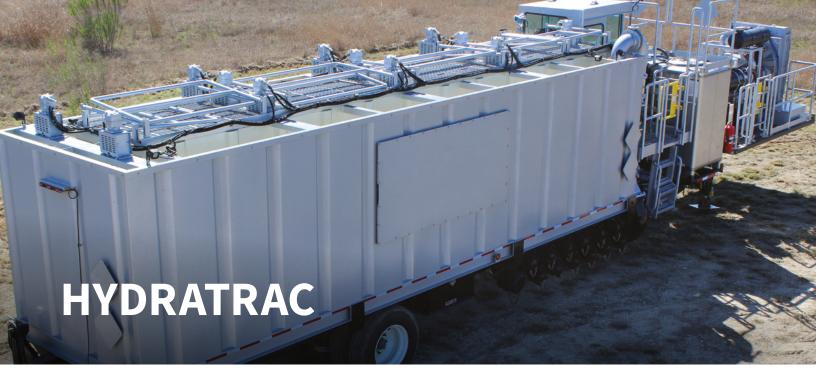
Our HYDRATRAC™ hydration controls system maintains tub level, pump speed, and controls up to eight chemical circuits.
