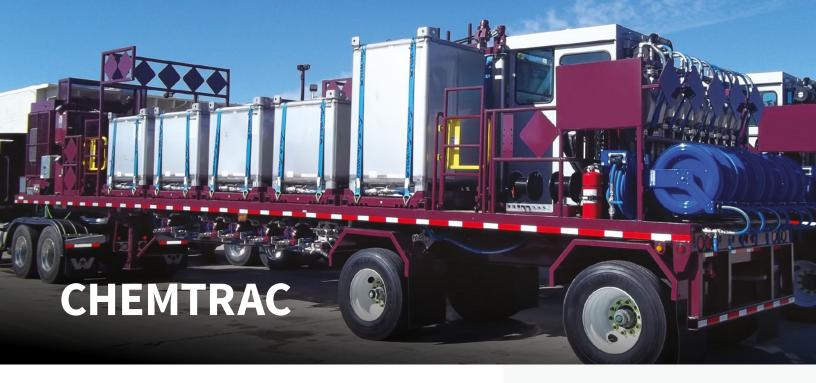
Our CHEMTRAC™ liquid additive system controls allow auto proportion chemical injection into your fracturing fluid.
