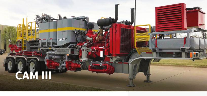
Rolligon CAM system is a continuous automated mixing control system designed for twin or single cementing pumping equipment. The system automates all aspects of the cement mixing process including mix water, bulk cement, and tub level. Combined with the industry-leading TEM™ mix head, the CAM system can accurately place cement in your wellbore.
