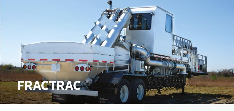
Our FRACTRAC™ blender controls system maintains tub level, pump speed, and controls up to eight chemical circuits.
