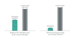
million pounds/645 metric tonnes. Larger-bore carbon steel pipes would have been required for the same throughput of water, so Pioneering Spirit would have needed 48-inch steel pipe, rather than 40-inch fiberglass pipe.
