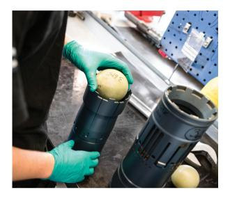
Our proprietary i-Frac CEM sleeve is a cost-effective, cemented, balldrop activated, multistage frac solution with a unique design that would ensure multiple fractures along the length of the well with up to five initiation points per stage.
