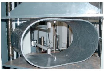
Before technical approval could be obtained from TUV, external loading capacity testing was performed:
