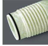
**SP/SPH** joints are 4 threads-per-inch with round form (SP) or buttress (SPH) profiled sealing threads. A secondary seal is provided by an o-ring gasket fitted within a groove in the male end. This exceptionally user friendly connection is used in high pressure applications up to 2,500 psi (17.2 MPa) and temperatures up to 212°F (100°C).
