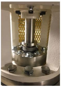
12MR seal aligned and set to proper spring load.
