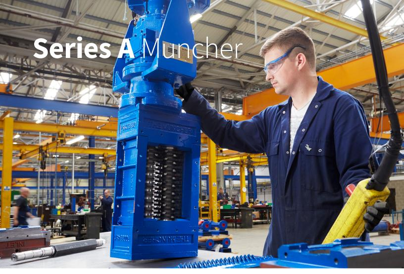
A high torque, low speed grinder for open channel and wet well installations suitable for the efficient disintegration of solids within a flow.
