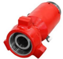
Anson top entry check valves are available with hammer union connections in sizes from 1 to 4 in., with working pressures up to 15,000 psi for sour service and 20,000 psi for standard service.
