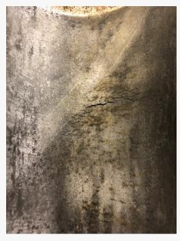
With presence of pitting throughout the coiled tubing's ID surface, the test sample still surpassed 100% predicted fatigue life.
