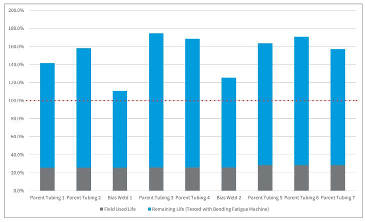
Compounding field used fatigue life as recorded by Cerberus™ suite with laboratory test data on the retired string, all samples including those containing bias welds surpassed the 100% mark of predicted fatigue life. Despite the presence of pitting, ATP-130 provides service companies and operators peace of mind while helping deliver full revenue potentials.
