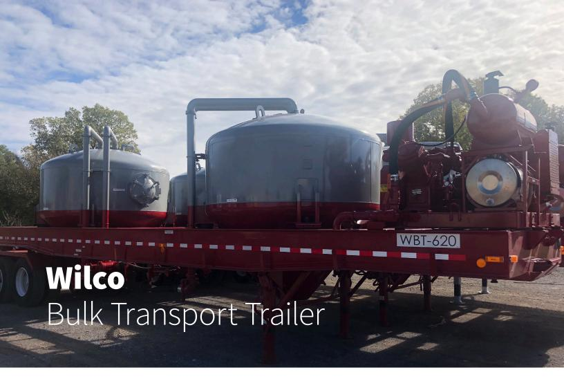
Wilco™ WBT-620 (620-ft³) and WBT-660 (660-ft³) bulk transport trailers are designed for rapid unloading of bulk materials. Versions are available with and without engine and compressor packages.
