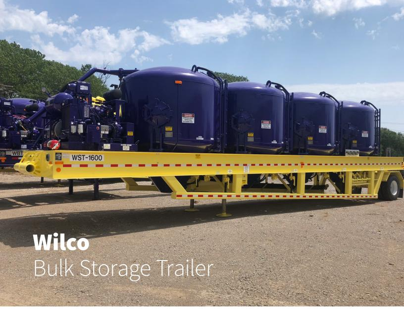
Our Wilco™ WST-1600 trailer-mounted stationary bulk storage bins incorporate four pressure vessels and are used for on-site storage and pneumatic-handling of bulk cement and other powdered bulk materials. The vessels can store up to 1,660-ft3 of bulk materials. The trailer is deployed to well locations empty. The trailer's hydraulic landing legs are contracted and the four-tank trailer drops to the ground where it is supported by a specially-designed under-frame structure.
