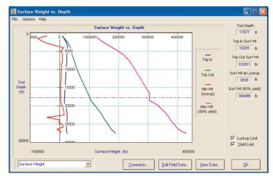
Cerberus for jointed pipe is a state-of-the-art software used for modeling any operation involving the running of tools, casing or completions into and out of wells. By analyzing the cumulative forces acting downhole at each stage of the job, Cerberus is able to determine whether the target depth can be reached, the desired tasks performed and the equipment safely returned to surface.
